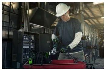
Tools in the new Next Generation line include 6-, 12-, and 15-ton crimping tools, as well as cable and bolt cutters, and a 10K PSI pump with removable heads that have the capabilities to do both.
